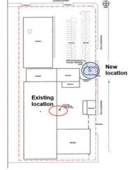
Mattco Forge produces engineered forged metal products for the aerospace, defense, oil and gas, transportation, and power generation industries. Mattco Forge is now applying to relocate an existing 499-gallon above-ground propane tank away from their entrances for safety purposes.
